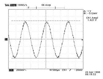
to the same level. These signals can be measured with an oscilloscope or an AC voltmeter. If you are using an AC voltmeter, remember that it reads AC signals as RMS values. In order to obtain an audio signal on P4, a valid COR or PL must be received. Once a valid access signal is received, the RLC-3 will un-squelch the audio and be present on P4.
