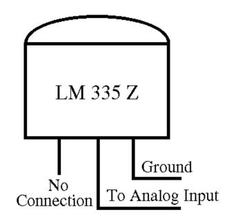
LM335Z Temperature Probe Connections Diagram
