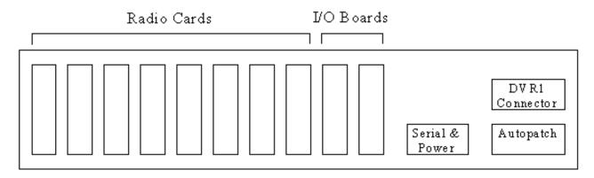
Each of the radio cards has two DB-9 connectors. The bottom one is used for connecting to a radio; it has connections for audio in, audio out, COR, PTT, and PL detect. We call this a radio port. Each radio port can be used for a repeater, a link, or a remote base. One of these radio port connectors will be used for the autopatch if you have one. The top DB-9 connector on each radio card is a serial port that can be used for controlling some types of remote bases.
