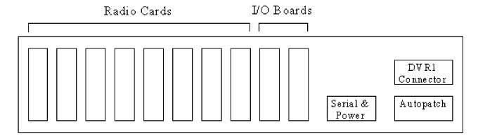
Each of the radio cards has two DB-9 connectors. The bottom one is used for connecting to a radio; it has connections for audio in, audio out, COR, PTT, and PL detect. We call this a radio port. Each radio port can be used for a repeater, a link, or a remote base. One of these radio port connectors will be used for the autopatch if you have one. The top DB-9 connector on each radio card is a serial port that can be used for controlling some types of remote bases.
