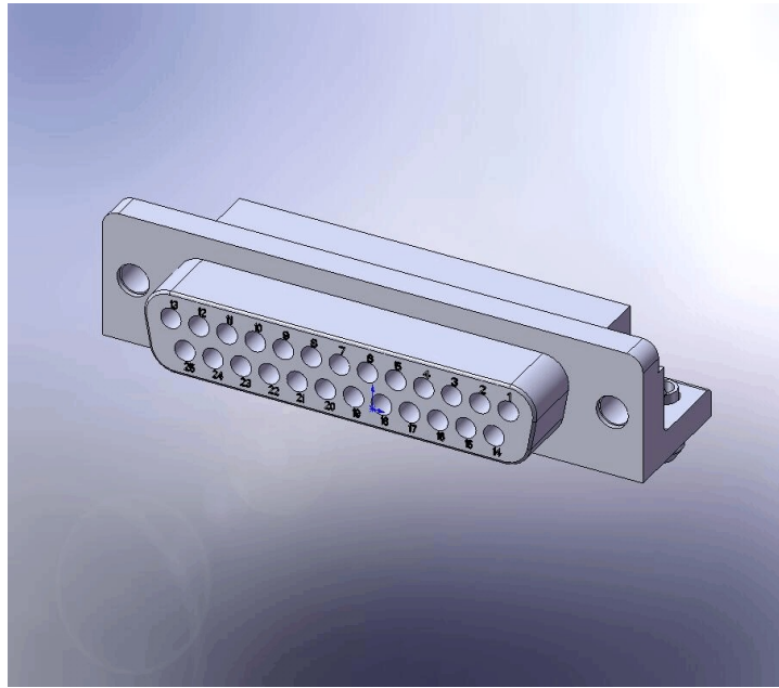
Front View of the DB-25 on the DSP-404
